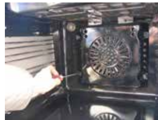
Take out the ventilation cover by loosen the screws
